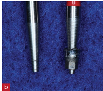
Figure 8: The retrieved fractured abutment fragment is shown on the retrieving instrument (a, b) and after separation from the retrieving instrument (c).
